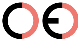
False CE Mark (too far)
